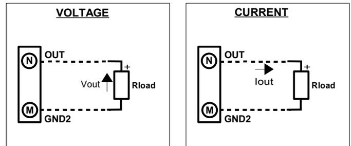
Note: terminal P = GND2; terminal O = Not connected (NC)
